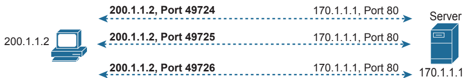
Figure 10-7 Three TCP Connections from One PC
