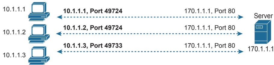
Figure 10-6 Three TCP Connections from Three PCs
